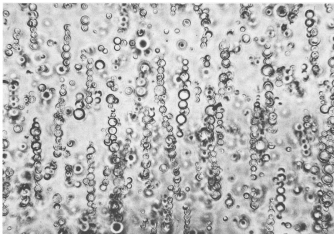
Fig. 1. Alignment of S. commune protoplasts by dielectrophoresis in an AC-field with a frequency of 2 MHz and a field strength of 100–130 V/cm
